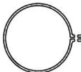
Bushing-Stinger Cover Cross-Section
